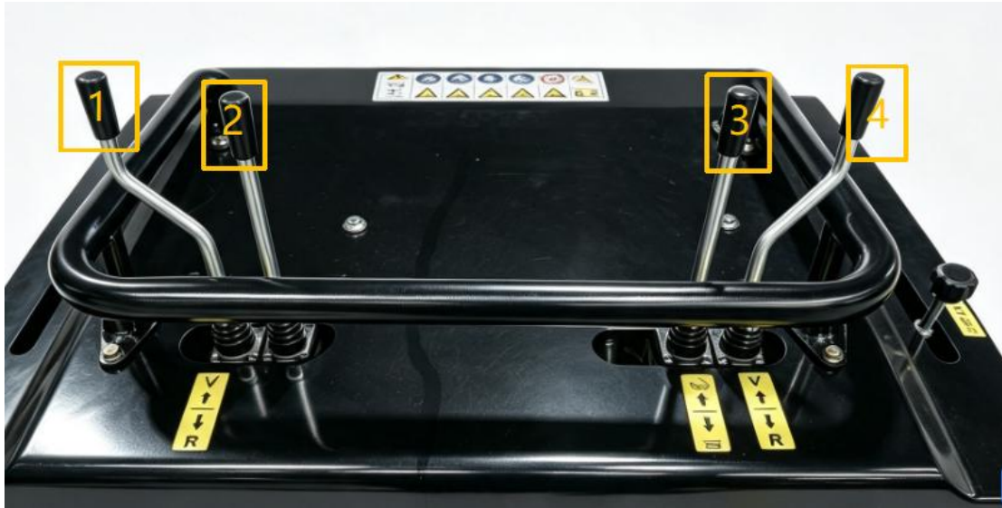
1-----Left track walking motion 2-----Hopper rotation motion 3-----Hopper unloading motion 4----- Right track walking action
